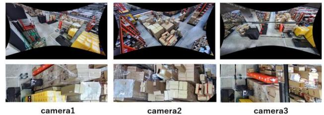
Fig.2. Captured Images from Three Cameras (Top) and Their Projective Transformed Images (Bottom) (Sample 1)
