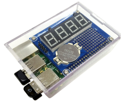
Figure 2. DF.sense (WiFi / BLE Scanner)
