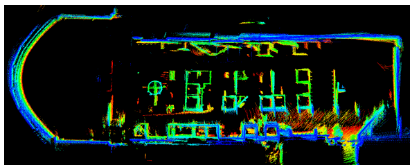
(b) Registered result with 350 frames. Colors indicate the altitude. (The roof and ground are removed for clearer show)
