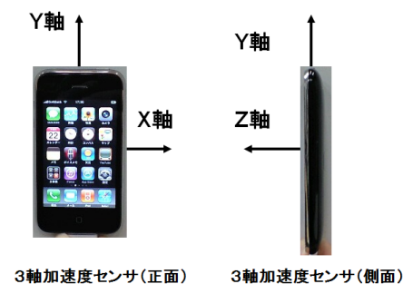
図1 加速度センサの軸 (iPhone) Fig.1 Acceleration sensor axis(iPhone)
