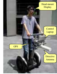
Figure 3. The segway can conduct moving wireless surveys both indoors and outdoors.
