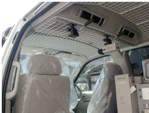
Figure 3. The interior of the DCV. Wire nets are attached for various arrangement of microphones.
