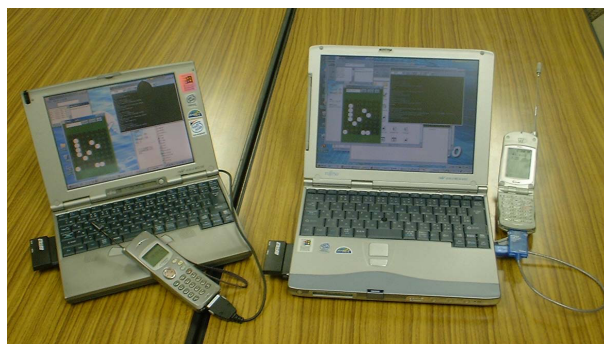
Figure 6: Ad-Hoc Communication System with Cellular Phone
