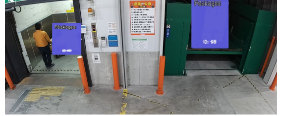
Fig. 6. Pallet detection and tracking with AI camera (left: elevator right: vertical transport system)
