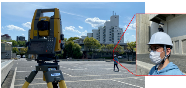
Fig. 1 An example of ToF/MFPS. TOPCON GT1205 is used for ground truth measurement [11].
