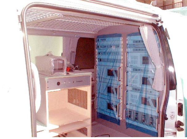
Figure 6: Recording Devices: six computers and network devices are built into the vibration-free rack.
