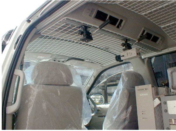
Figure 3: Ceiling: There are wire nets for attaching microphones
