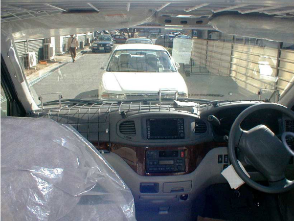
Figure 2: Front panel: There are wire nets for attaching microphones
