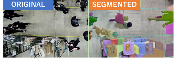
Fig. 12. Example of the segmentation in the warehouse using SAM
