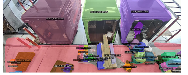
Fig. 5. Example of the recognition using instance segmentation
