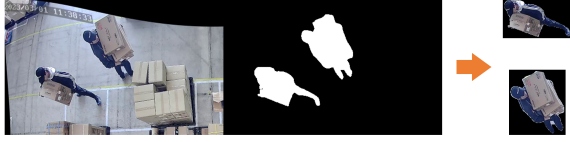
Fig. 8. Example of the segmentation using optical flow
