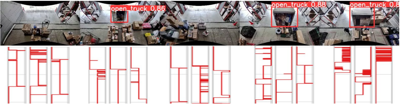
Fig.8. Recognition and visualization of truck berth status. Bottom graph is a time series of status (empty, close_truck and open_truck).
