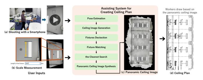
Figure 1: Assistance Method for Creating Ceiling Plan Using a Video from a Smartphone. The system synthesize (c) a panoramic ceiling image from 2 inputs of a user: (a) a video shot by a smartphone and (b) a scale measurement on the provided image. Users can draw (d) a ceiling plan accurately and quickly based on the synthesized image.
